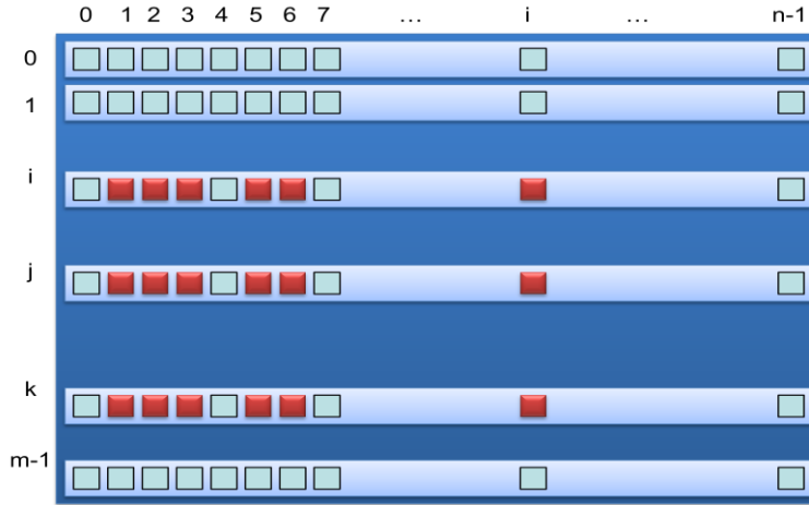
Fig. 4: Operating on selected components of the vectors. The operation \text{vect}_j = \text{vect}_i \text{ OP } \text{vect}_k is applied only on the selected components.
