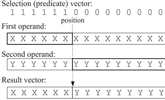
Figure 1: Parallel one-point crossover using predicate vector.
