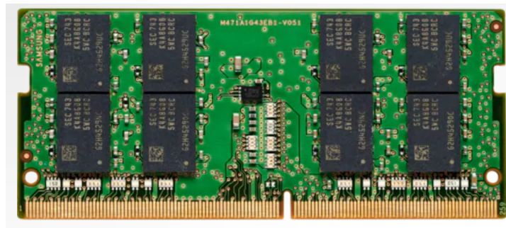
Figure 2.3: HP - DDR4 - 16 GB - SO-DIMM 260-pin.
